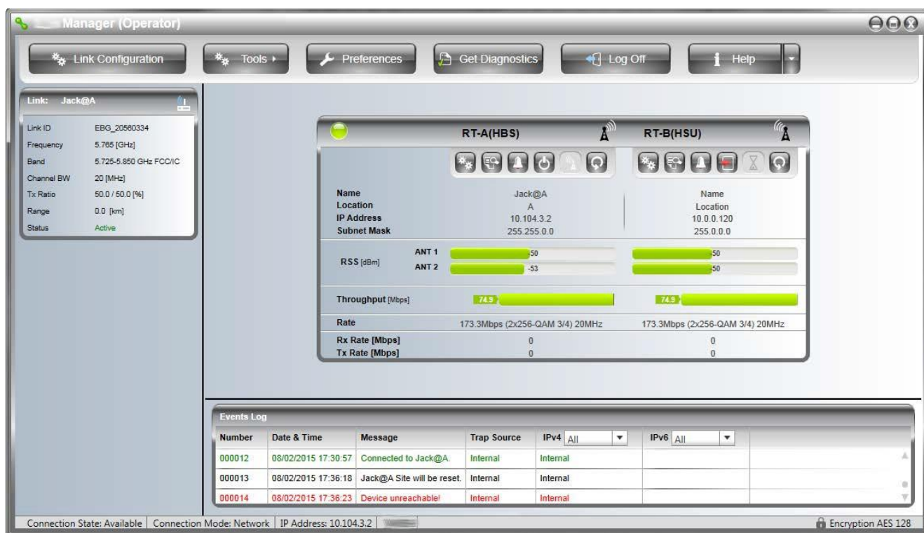
Figure 3-3: Main window: Link Master ODU activated, Slave ODU registered
