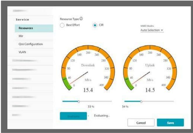
After the initial evaluation, dynamic monitoring of the sector is maintained. This allows you to add SUs in the sector, and the available resources are adjusted automatically.
