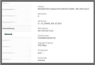
Dying Gasp on RT-B(HSU): Inactive: Low PoE voltage
