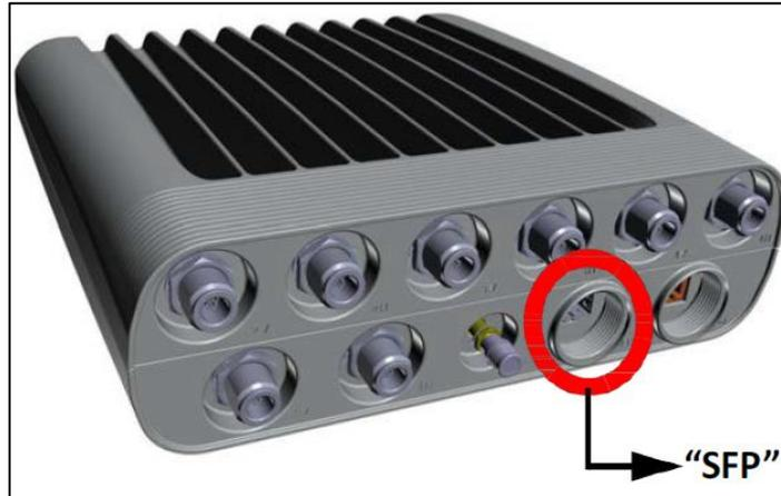
**Figure 95: Data port: MultiSector Base Station Connectorized**
