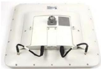
Connect cables to Turbo Gain
