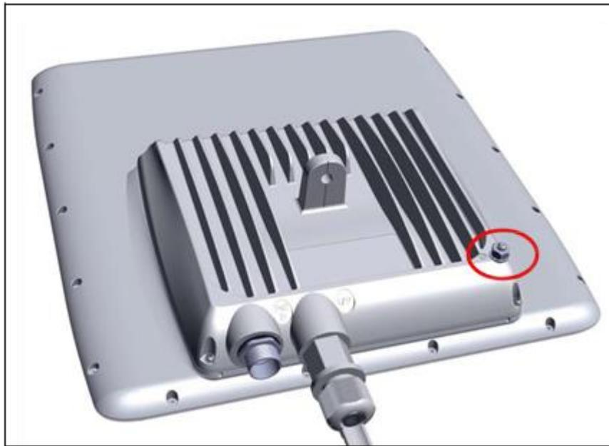
Figure 71: Ground: JET radio unit
