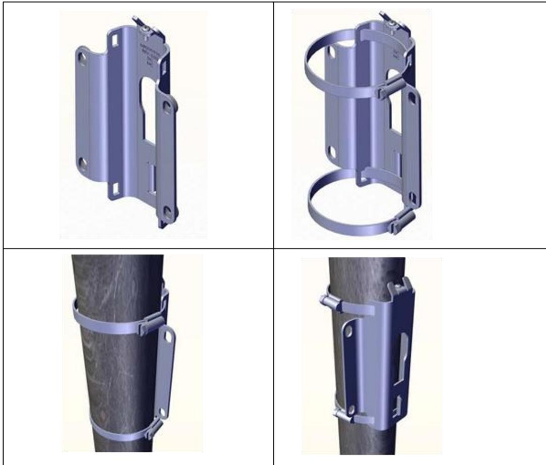
2. Place the mounting tongue of the MultiSector Base Station Connectorized in the indicated hole of the supporting mount, while aligning the vertical channel of the unit with the flange of the supporting mount. Make sure the MultiSector Base Station Connectorized is attached firmly to the mount:
