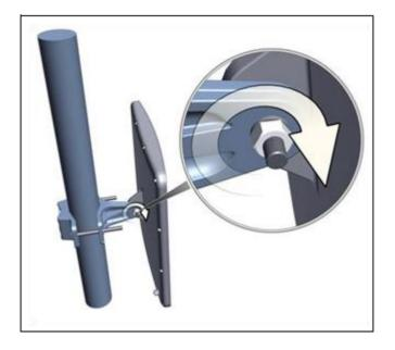
Figure 111: Tighten bolt (SU Integrated shown)
