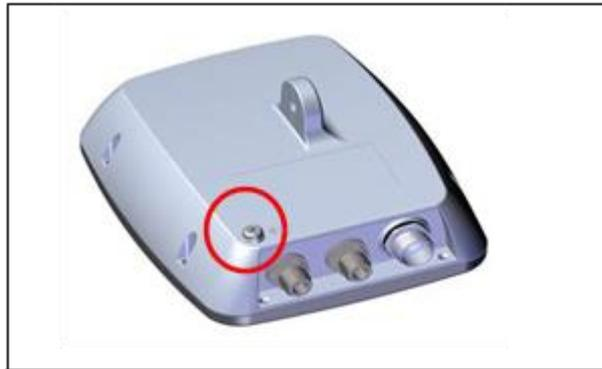
Figure 69: Ground: SFF radio unit
