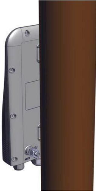
2. Fasten the unit to the pole using worm-drive clamps.
