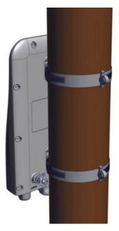
Figure 67: SU Connectorized mounted with worm drive clamps
