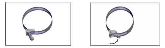
e. Once the band is at the correct radius, close the clamp and tighten with a screwdriver (make sure the tops of the screws face away from the mount):
