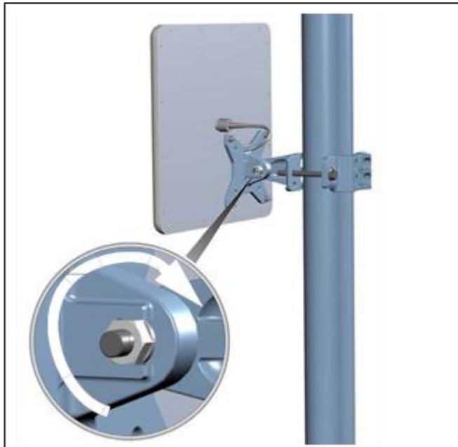
**Figure 112: Tighten bolt (external antenna for the SU Connectorized shown)**
