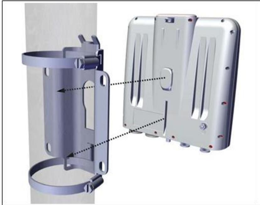
3. Push down on the MultiSector Base Station Connectorized until you hear a click, then fasten the locking screw as shown (the locking screw is found on the mounting tongue):
