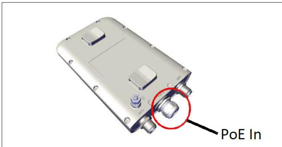
**Figure 25: Laptop/network port: SU Connectorized radio units**
