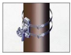
c. Slide the metal band through the clamp:
