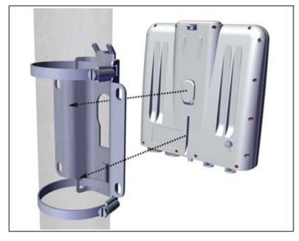
3. Push down on the MultiSector Base Station Connectorized until you hear a click, then fasten the locking screw as shown (the locking screw is found on the mounting tongue):
