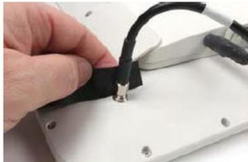
Sealing tape for Turbo Gain
