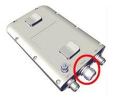
Figure 89: Input port: SU Connectorized unit ("PoE In")
