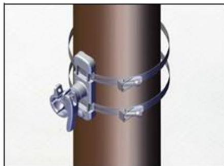
c. Slide the metal band through the clamp:
